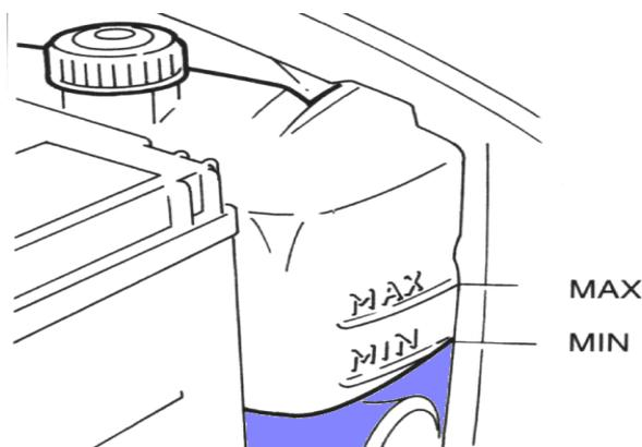
Check the coolant level in the reservoir tank when the engine is cold. If the coolant level is below the "MIN", add coolant up to the "MAX" level.
